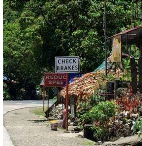
Figure 16. Imprecise Arrangement of Traffic Signs
